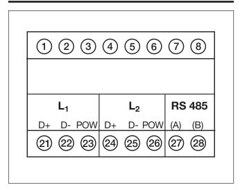
Use 3\*1,5mm2 single core wire for  $L_1$  and  $L_2$  bus Use 2 wires with shield for the RS485 connection (Distance up to 1200 Meter)
